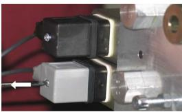
5. Remove the UP solenoid plug (grey) on valve
