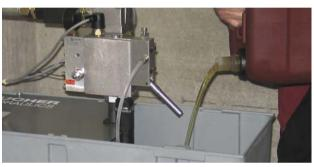
3. Fill with hydraulic oil to 40 mm below the cover
