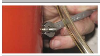
7. Unscrew air-bleed screw on cylinder head by one turn
