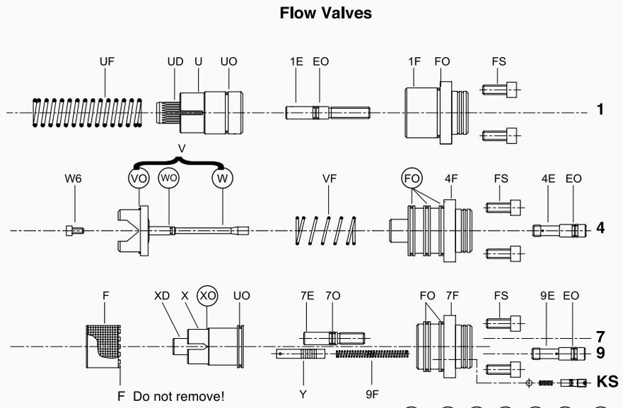
In case of down leakage, replace and test in the following order: (DS) & (DN), (XO), (VO), (WO), (FO) + (HO).
