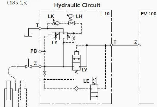
**Rest Position:** When L10 is at stand-by, the solenoid LE de-energized and the main flow guide LV closed, preventing flow from cylinder to tank.
