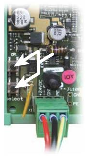
1. On the Handterminal select menu 3, then "Adjust./tests", then "Pipe rupt. test"
